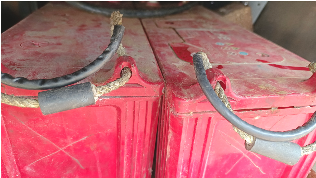
Example of Accessible MF (left) and Full Sealed MF (right) batteries fitted on a truck. These are 120Ah batteries, commonly called N120.
