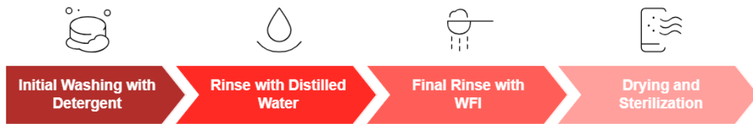
Figure 10.2 Cleaning and washing process
